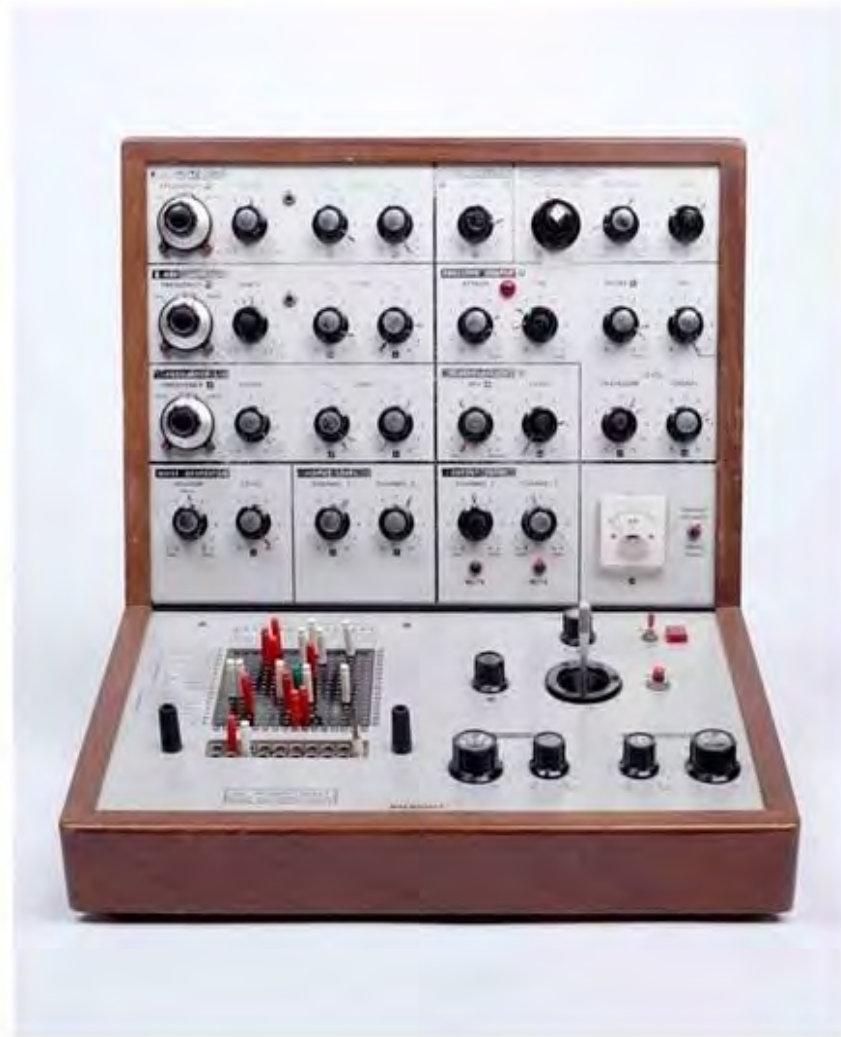
Elevated front view of The Putney (VCS 3). Afromos (African task) chassis housing aluminium control panels.
