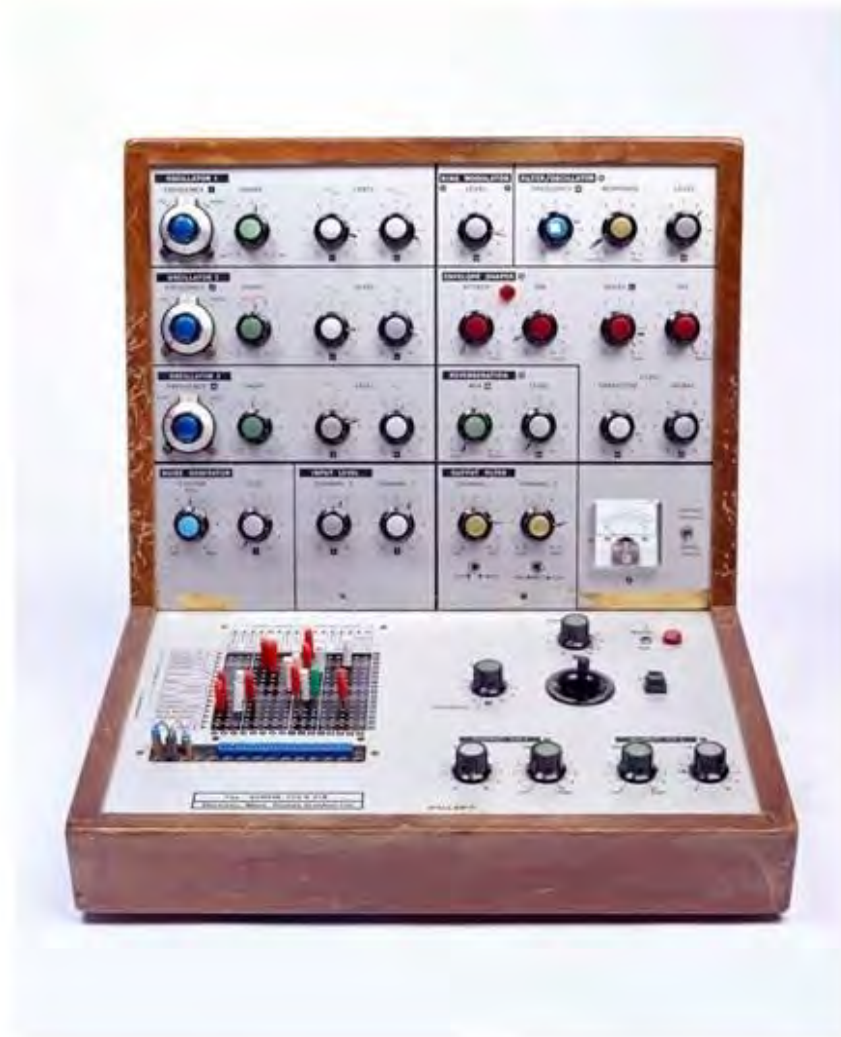
Elevated front view of The Synthesis (VCS 3). Afromos (African task) chassis housing aluminium control panels with colour-coded oscillators and controls.
